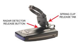
2 - Push the RD Release button and slide the RD onto the Spring Clip until the RD hits the bottom of the Tab. Then release both the Tab and the Button. Now slide the RD toward you until you hear it lock into position. Remove the RD a few times so you can observe how the spring clip functions. When used properly, the spring clip avoids putting excessive pressure on the mirror stem when installing and removing the RD.
