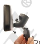
3 - Install this mount from the passenger side of the vehicle. Remove the right half of the mount by removing the two socket head cap screws. Be aware that there is a small lock washer on the lower screw. With the left half of the mount still attached, position the mount around the mirror stem as shown above.
