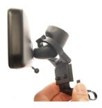
4 - Reattach the right side of the mount. Make sure the small lock washer is still on the lower screw and tighten untill the screw is fairly snug. Leave the top screw loose so the mount can slide towards the windshield around the large diameter of the mirror stem.
